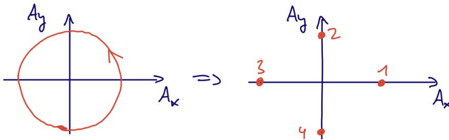
That is, we assume that the field is kept constant over quarters  $T/4$  of the driving period  $T$ , and points along positive and negative  $x$  and  $y$  directions as sketched, with an amplitude  $A_0$ .
